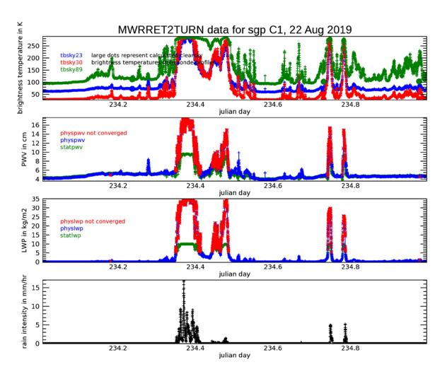
**Figure 6.** Quicklook image of MWR3C measurements and retrieved LWP and PWV on 22 August 2019 at the SGP C1 site.
