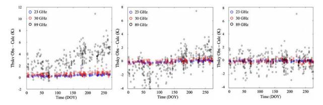
**Figure 1**. Brightness temperature residuals ( $\Delta T_b$ ) recorded at the ENA site in 2017. Uncorrected values are shown in the left panel, annually corrected value (based on a single set of bias offsets for the entire year) are in the middle panel, and monthly corrected values are in the right panel.
