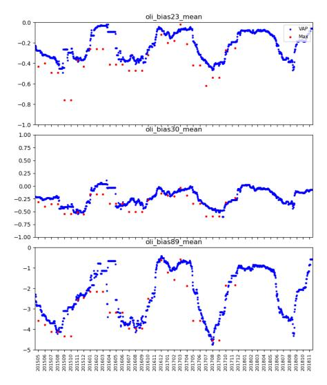
**Figure 3**. Comparisons of mean  $T_b$  bias at the three frequencies from the automated technique with manual monthly  $T_b$  bias at the Oliktok Point site (Max).
