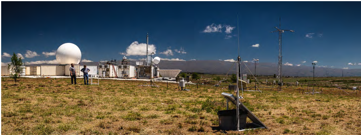
Figure 3. The primary instrument cluster for CACTI during the first ARM Mobile Facility (AMF1) deployment in Argentina. In the background is the Sierras de Córdoba mountain range that contribute to frequent strong deep convection in the region.
