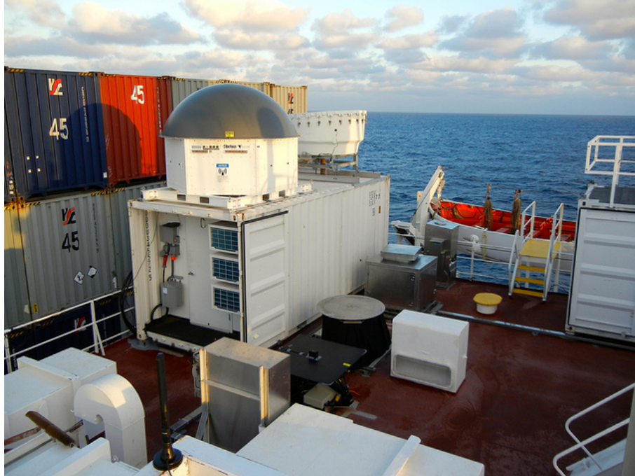
Figure 4. The second ARM Mobile Facility deployed on the Horizon Spirit for a marine boundary layer cloud experiment in the Eastern Pacific.
