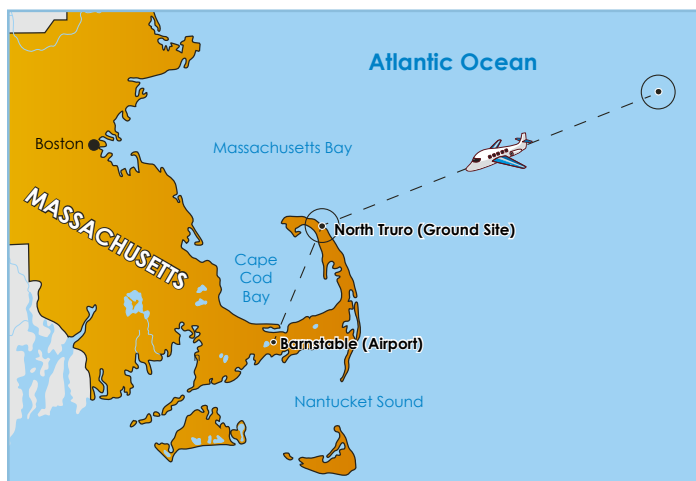
For TCAP, instruments are measuring one “column” in the sky above the ARM Mobile Facility site in North Truro, Mass., and another “column” out over the ocean, about 155 miles off the coast.
