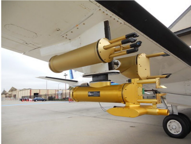
Figure 6. Instruments mounted under G-1 wing.
