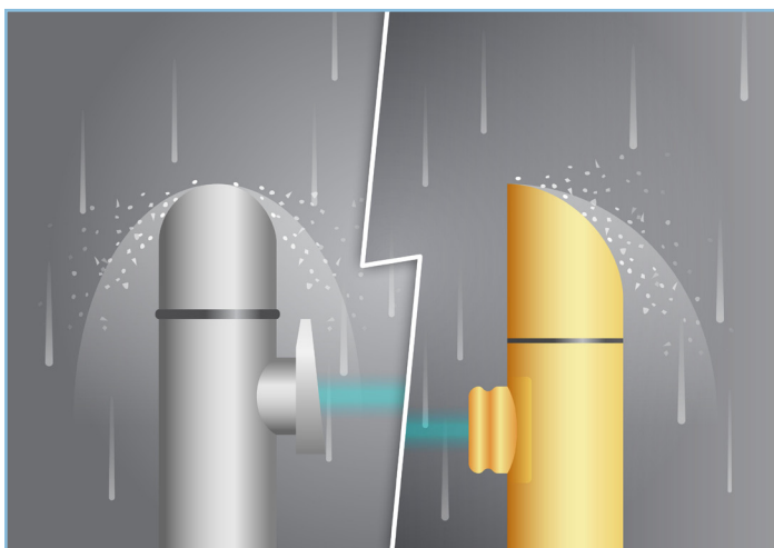
Newer aircraft probe designs could minimize the shattering effect that previously resulted in a disproportionate amount of smaller particles being measured by the sensor beam.
